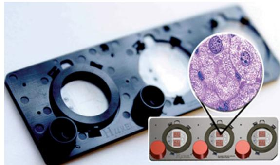
The H $\mu$ RELflow™ cell-based assay system has three microfluidic devices on a biochip. Each device incorporates two cell culture compartments interconnected by microscale canals. Integrated micropumps recirculate culture media within the device.
