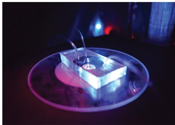
The microfluidic system shown above has been used by Florida State University researchers to deliver glucose to islets of Langerhans, the endocrine portion of the pancreas. The researchers used laser illumination to measure hormone release and assess the response to varying glucose levels.
