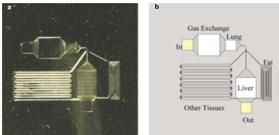
Figure 1 a) Photograph of a four-compartment Hurel, b) schematic diagram of this chip. This four-compartment Hurel was fabricated in silicon using standard microfabrication techniques. In this example, there is a liver compartment, a fat compartment, a lung compartment, and an other tissues compartment.
